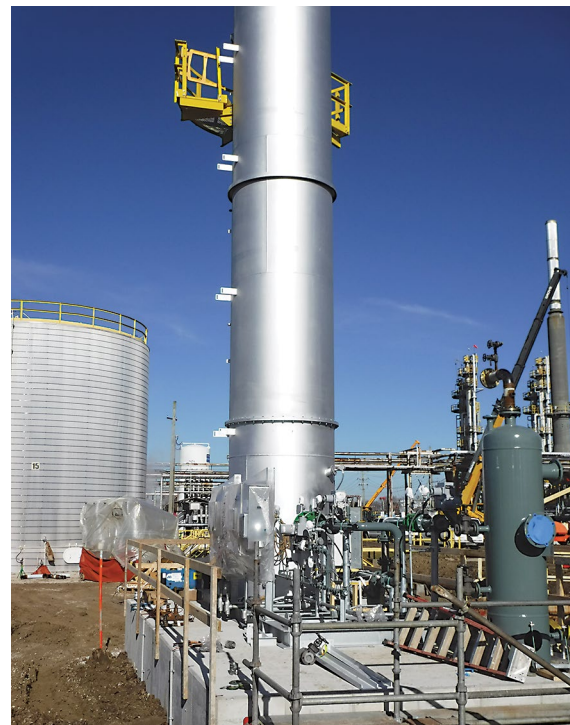
The new Vapor Combustion Unit (VCU) that will be used to burn off the vapors displaced when loading gasoline and diesel into railcars.
